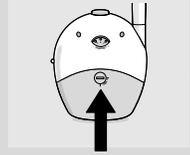
**1** Remove the battery compartment cover using a coin.
